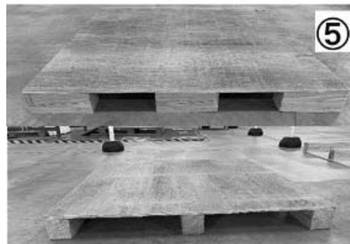
Fig.7 Condition of floorboard after test (1st exam)
