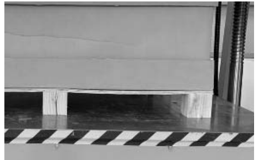
Fig.11 Condition of floorboard after test (2nd exam)
