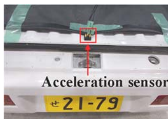
Fig. 2 Acceleration sensor installed on the vehicle bed
