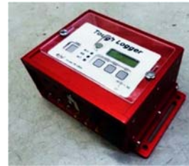
Fig. 28 Transport environment recorder tough logger (TR-1000, IMV Corporation, Japan)
