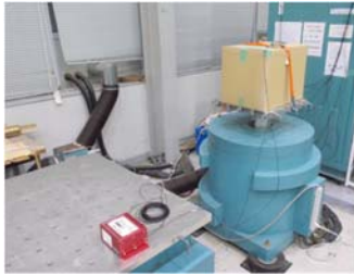
Fig. 25 Dummy packaged product fixed on top of the vibration table
