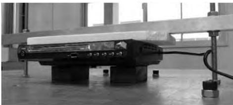
**Fig.7 Sample and supporting method.**
