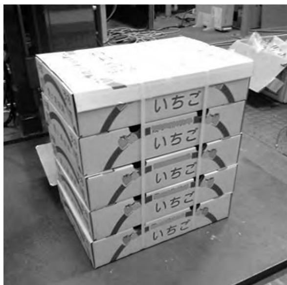
Fig.2 Form of packaging for estimation of peak acceleration ( PA_{cc} ), velocity change ( V_c ) and fruit damage.
