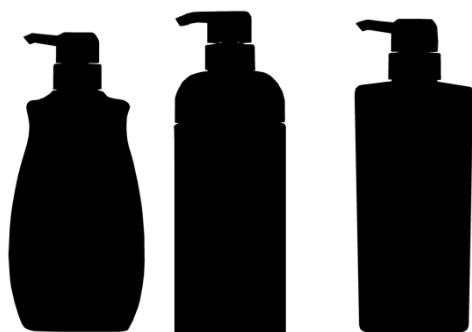
Fig.1 Binarized frontal view images of liquid soap bottles (Sample A, B and C)
