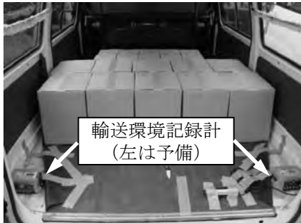
Fig.1 Vibration measurement of carrier during transportation
